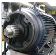
1. Position hub on motor shaft
