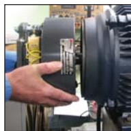
2. Place brake on hub, no disassembly required
