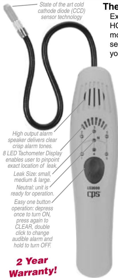
State of the art cold cathode diode (CCD) sensor technology
